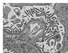
Specimen: ultra thin section of mouse kidney (contrast reversal) Accelerating voltage: 5.0 kV Scan speed: 0.04 \mu\text{s}/\text{pixel} (S, 120 \times 3,840)
