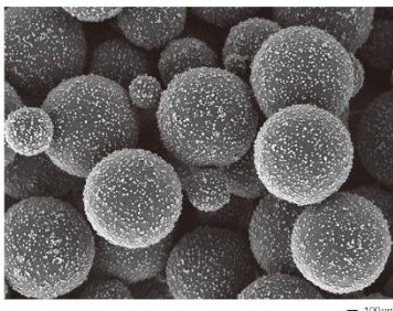
Specimen: Acrylic particles Accelerating voltage: 0.7 kV Observation mode: BD Detector: UI ID
